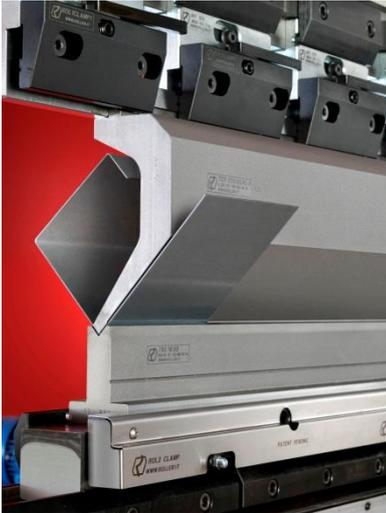
Picture 2-Press brake tooling
